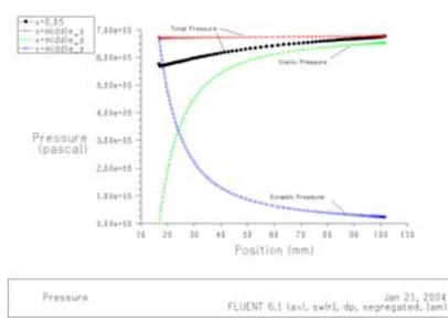
Figure 8.: Pressure distribution along radius, laminar solution.
