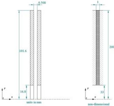
Figure 3.: Geometry for one gap 2D model.
