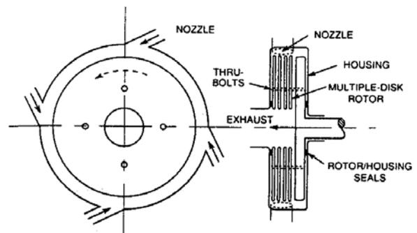
Figure 2.: Schematic diagram of Tesla turbine [2].
