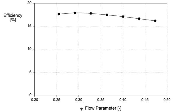
Figure 15.: Efficiency for turbulent solution, isolated disk.
