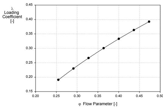
Figure 9.: Characteristic curve, loading coefficient, from laminar case.
