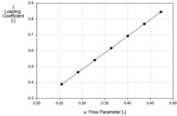
Figure 14.: Loading coefficient for turbulent solution, isolated disk.
